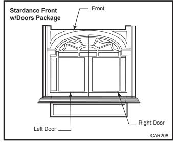
Fig. 2 Carton contents for operable door package.
